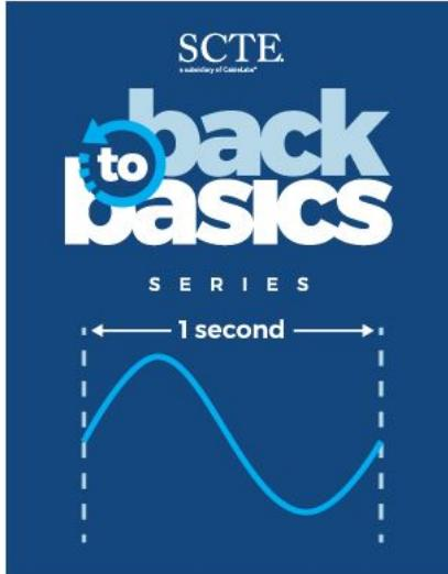
Frequency is the number of times — typically per second — that a repetitive event happens. For an electromagnetic wave, frequency is the wave's rate of oscillation. Commonly measured or stated in units of hertz (Hz), which is the number of cycles per second
